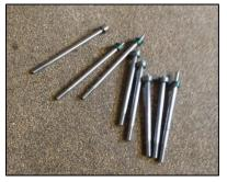
1/8 shaft that has a 5 BA threaded section .406 long and plain shaft at 1 3/4 long, I machined an extra small spigot to the end of this to locate the top on. The top was again a simple turning job with overall dimensions of 7/32 diameter and 3/32 height plus a central hole to fit the spigot on the shaft, I machined the top to size once it had been silver soldered to the shaft. Picture shows the two parts waiting silver soldering.
