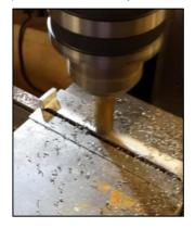
Once they had been tidied up a little, they both had their ends machined square until they were exactly 4" across, the picture then shows the rear stay being machined down in thickness to the 2 mm shown on the drawings although I left the ends a little thicker for more strength.
