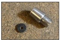
wood with the No.29 using a power drill. To begin with I did this the other way around, drilled the rubber, placed the tool over with a length of 1/8 BMS to line up and then tapped the tool with the hammer but had a tendency for the hole to end up off centre so changed the order of doing things which worked very well.
