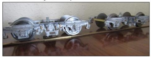
the supplied bits so I have just made them up as JVR type bogies with PTFE bearings and they seem to roll very well. There is an opportunity to add a few bits of detailing for the spring supports on the castings which you can see I have done with Brass rod.
