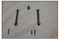
7/32 AF hex, a 3/16 ball machined on the bottom to fit the recess on top of the axle box and the threaded section above to fit it to the spring yoke. I have modified the cup a little, first it has a N0.54 hole through it and the bit threaded section I beefed up (for strength) to 4 BA instead of 6 BA to allow for the small bore going through it. This is for the oil to pass through, you won't see it for a while, but later
