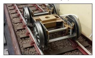
the guard irons. I later changed the way that the irons are bolted to the frames just to make things more practical. I haven't set the springs yet in this picture, it's probably best to do this once the loco is close to completion or at least after the boiler is sitting on its frames.
